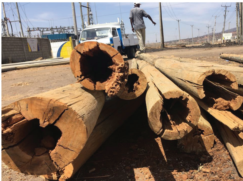
The bane of Kenya Power: badly treated poles, the inside having been devoured by termites because of poor treatment. Photo G. Muthike
